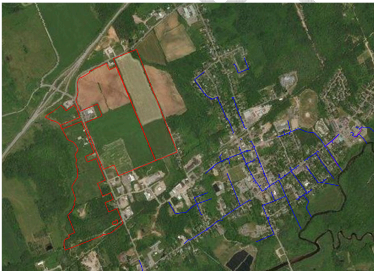
Figure 2-5 Stormwater Sewer System and Properties of Interest
